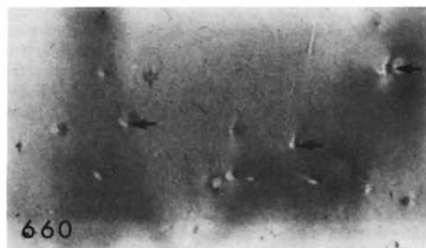
Fig. 3. Lang-type topographs of a monochromator with 500 \mu\text{m} thick wafers and Mo K\alpha_1 radiation. The \theta -offset was to half-height on the central double-crystal rocking-curve correlation peak in each case. Field 12 \times 6 \text{ mm} .
